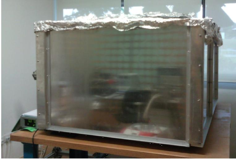
Figure 10: Picture of the bakeout process. The vacuum system is contained within this large metal cage as temperatures are raised to between  $150^{\circ}\text{C}$  to  $200^{\circ}\text{C}$ . The mechanical pump is running continuously as the air inside the chamber is being evacuated. The process takes place over the course of approximately 2 days.
